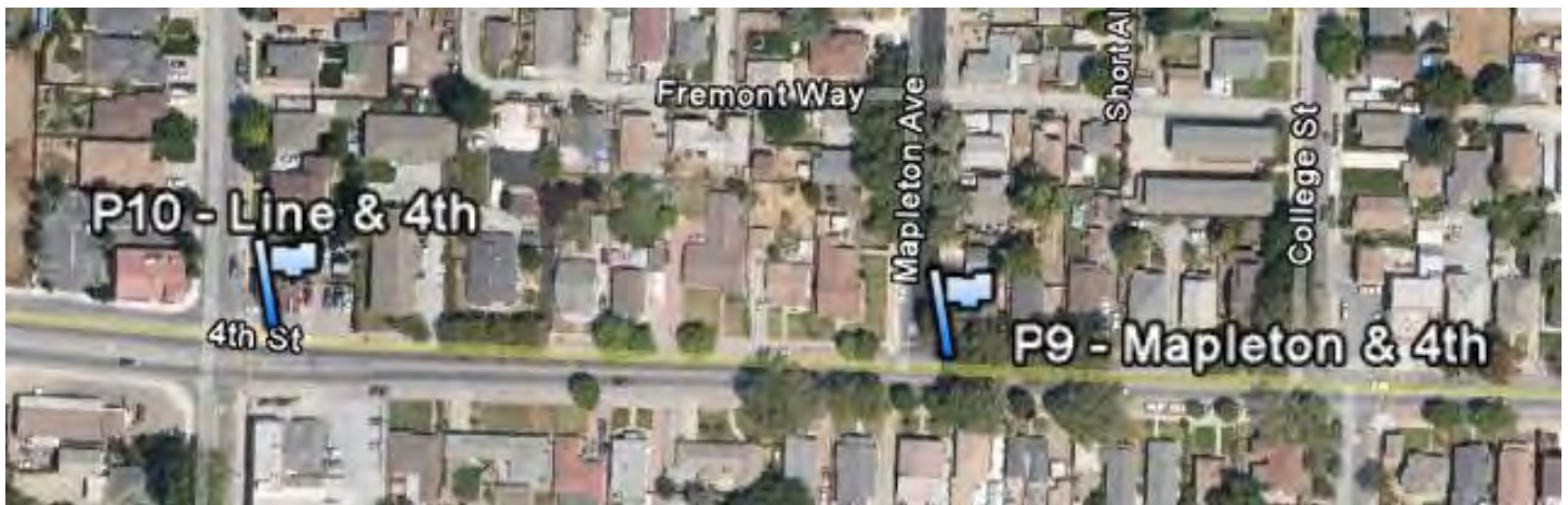
The north side of 4th floods at Mapleton and continues flooding to west to Line St. Very flat gutter (0.2%), tree roots and bulging driveway block the flow to west in gutter. Storm drain inlets are located at Line & 4th.
